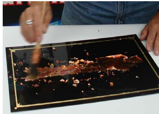
After the gold leaf is applied brush away the excess with a soft brush.
