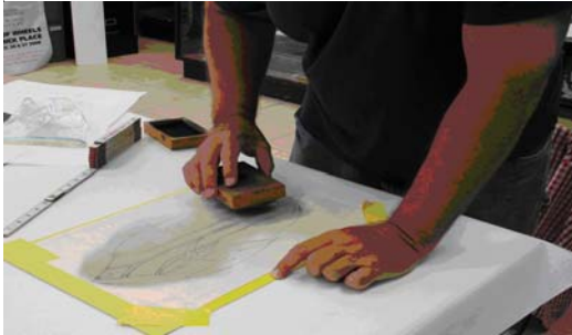
Above I am pouncing the pattern onto the paint mask.
